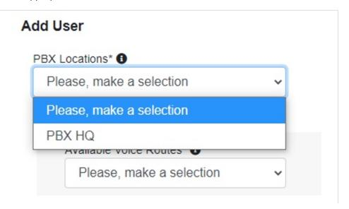
19. For each CrexendoVIP user created there will be an option to use an existing endpoint on the PBX or to create a new one. Upon selecting the SIP user from the dropdown, all existing devices registered to that user will populate. Here you should see the new phone we created that ends with T, for example 100T. Here is a preview of the screen and what we will be editing.
